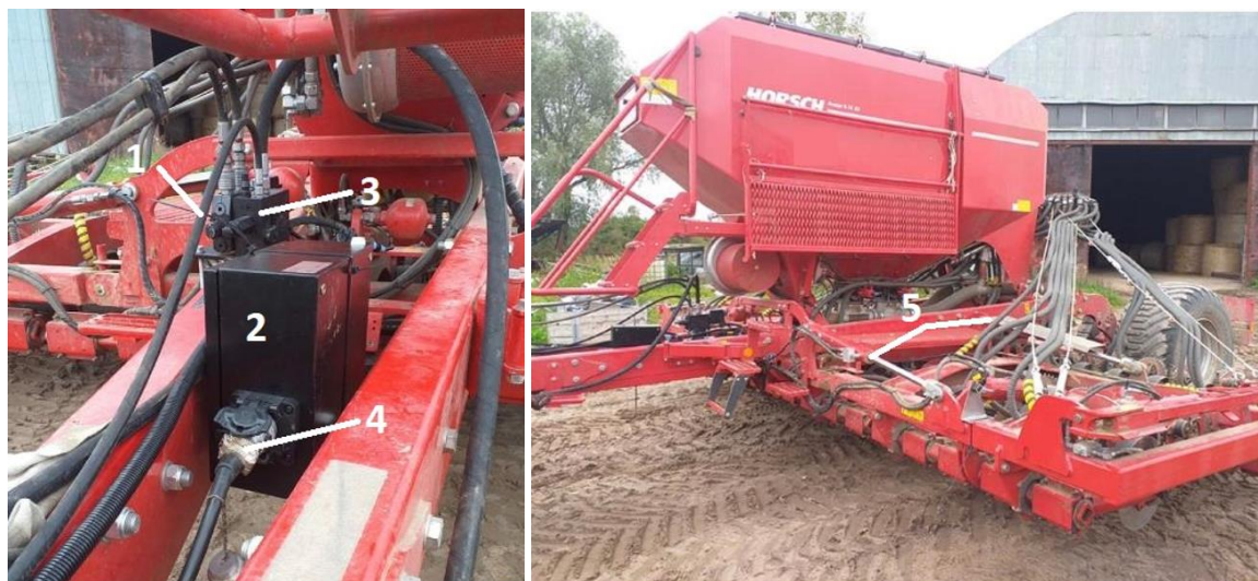
Fig. 1. Seeder with additional equipment for changing the seeding depth: 1 – hydraulic hose; 2 – ISOBUS control module; 3 – hydraulic block; 4 – ISO standard connector; 5 – two-way hydraulic cylinders
